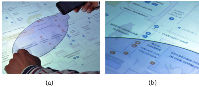
Figure 110: Personalized interaction example 2: IdLenses allow users to view content on an interactive surface through a customized view [16].
