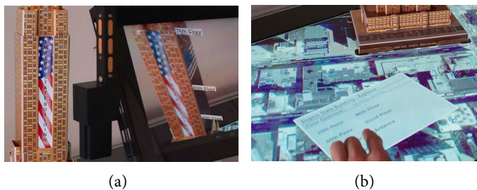
Figure 77: Augmenting physical objects with spatially registered annotations (a) allows users to select and explore diverse points of interest (b) that are then presented through the tablet.
