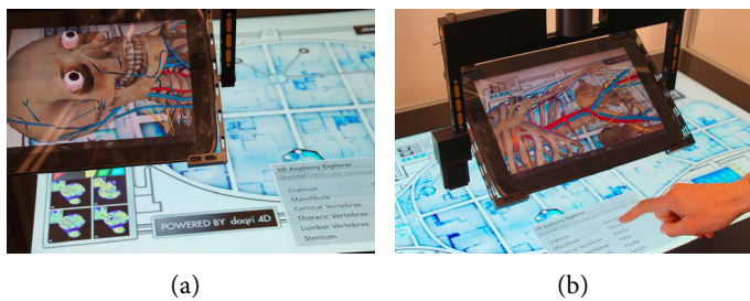
Figure 80: The anatomy explorer allows users to explore, for instance, the human skeleton (a) by selecting bookmarked bones from a list (b) which triggers the tablet to move to that position.
