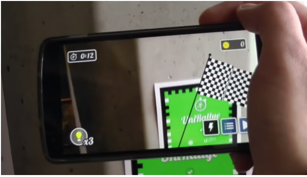
Fig. 3. The UniRallye interface displaying a destination flag AR element at the final target of a navigation task.
