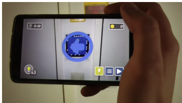
Fig. 2. The UniRallye interface displays a navigational hint in the form of an AR arrow element upon detection of the corresponding AR marker.
