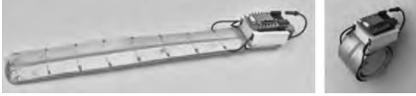
Figure 2. The SnapBand -prototype in a flat (left) and curled (right) configuration. A BLE Nano at the end of the band serves as a micro controller powered by a CR2032 coin cell battery.
