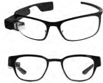
FIGURE 5.3: Google Glass (top), as announced in 2013, including optional glass frames, and Focals (bottom, © by North [138]), as announced in 2018, as an attempt to more closely resemble conventional eyeglasses.
