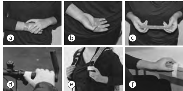
Figure 1. SnapBand is a touch input device that can be snapped, worn and attached to multiple on- and off-body locations, such as onto the wrist similar to a smartwatch (a), as a one- or two-handed touch controller (b&c), attached to a handlebar on a bicycle (d), on a strap of a backpack (e) or the edge of a table (f).
