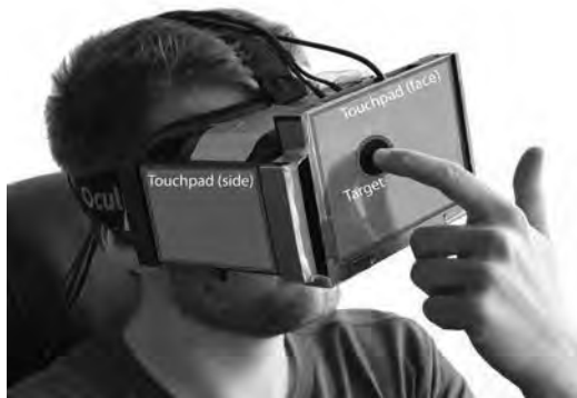
Figure 3. The FaceTouch prototype. A capacitive touchpad is embedded into a 3D-printed case and attached to the backside of an Oculus Rift DK2 via 5 small buttons that allow for pressure sensing on the touchpad. The side touchpad was only used in the second user study and does not have any buttons attached to it.
