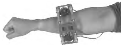
FIGURE 6.4: Positional feedback on the user's forearm using a self-actuated wearable. Pub. VII.
