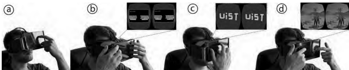
Figure 1. (a) A user interacting with FaceTouch , a multi-touch surface mounted on the back of a VR HMD. FaceTouch allows for precise interactions which can be used to implement applications such as text entry (b) or 3D modeling (c). Leveraging the sense of proprioception a user is able to blindly interact with control elements such as used in a gamepad to control a shooter game (d).
