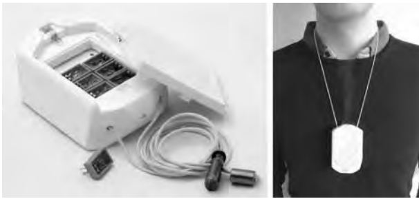
Figure 3. Left: The inScent prototype with opened top lid. Up to 8 scent cartridges can be plugged in. Each cartridges contains highly viscous scented liquid soaked into glass fiber to deter leaking. Right: Normally, scent emission is not visible to the eye. For this photo, we highly increased the amount of glycerol to make the scent emission visible as smoke.
