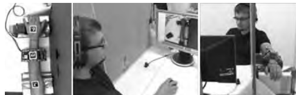
Figure 4. (Left) Marker-based camera tracking of movement and positioning. (Center) A user estimating and marking the Movelet ’s position on a previously taken image of his empty forearm, (Right) while his left arm wearing the device is hidden behind a visual cover.
