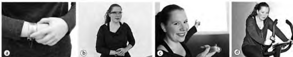
FIGURE 5.13: The SnapBand as a touch input band (a) that can be snapped, worn and attached to multiple locations, e.g. at the wrist to serve as an input device for smart eyewear (b), held in the hand as a tool for presentations (c), or attached to the handlebar of a gym machine for an easier reachability during a workout (d). Based on Pub. V).
