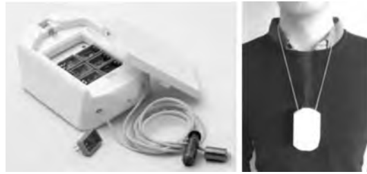
FIGURE 6.8: (Left) inScent is a miniaturized wearable olfactory display that contains up to 8 cartridges with varying scents for mobile notifications. (Right) The device is worn on a necklace. For scent emission, scented air is blown towards the user's nose. (For this photo, the airflow was made visible by adding glycerol for smoke). Pub. VIII .
