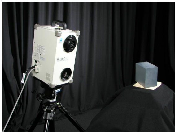
Figure 1. The setup used for test scans consisting of a Minolta VI-910 laser range scanner and the 90° calibration target.
