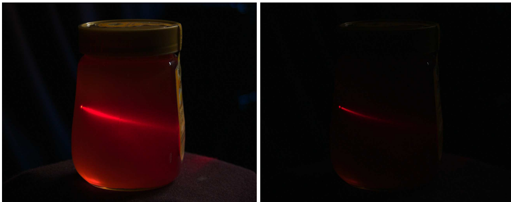
Figure 2.1: Example for single scattering inside an object. Left: A glass of honey illuminated with a red laser beam. Right: Shorter exposure time in order to improve visibility of the laser beam.
