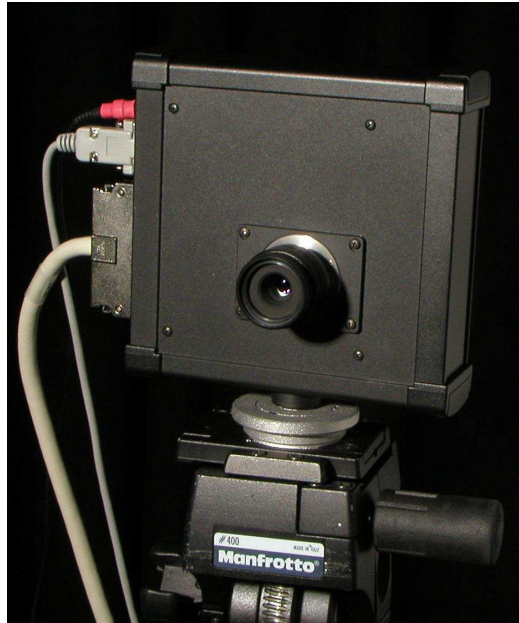
Figure 4.7: Photograph of the Silicon Vision Lars III high-dynamic range video camera
