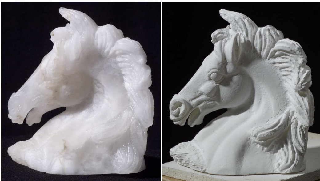
Figure 1.2: Photographs of an alabaster horse model with and without subsurface light scattering under identical lighting conditions. Left: Original object, much surface detail is hidden by the translucency. Right: The object is covered with fine white dust to stop light from entering the object.
