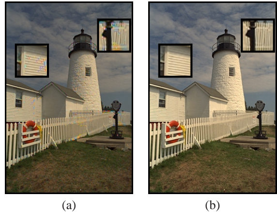
Figure 2. a) Applying the AAI algorithm to Bayer CFA data vs. b) applying the AAI algorithm for red/blue color channels to the image with perfect green channel. Notice how the AAI red/blue channel interpolation creates an almost perfect image.
