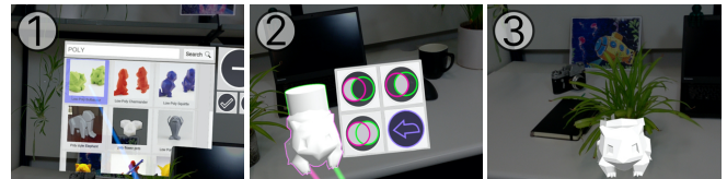
Figure 11: In-Situ remixing of a figure to create a planter. Searching for a base design (1), placing the components (figure and cylinder) and applying subtraction (2), visually verifying proportions (3).
