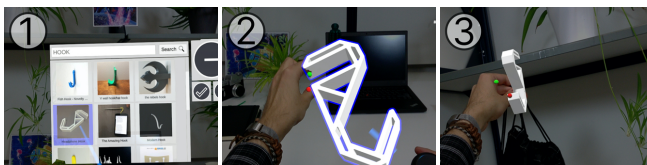
Figure 13: Choosing and altering an existing design. Browsing through hook designs (1), scaling of a fitting one (2), in-situ verification that the hook would be mounted high enough (3).
