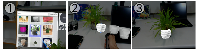
Figure 10: Adaptation of a fitting planter design to the existing plant. Browsing (1), comparing alternatives (2), customizing / scaling to fit (3).
