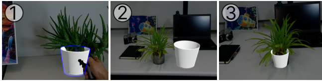
Figure 12: Replicating an existing physical artifact (planter). From left to right: Copying the mesh (1), previewing the result in terms of size (2), correcting the scale and proportions (3).
