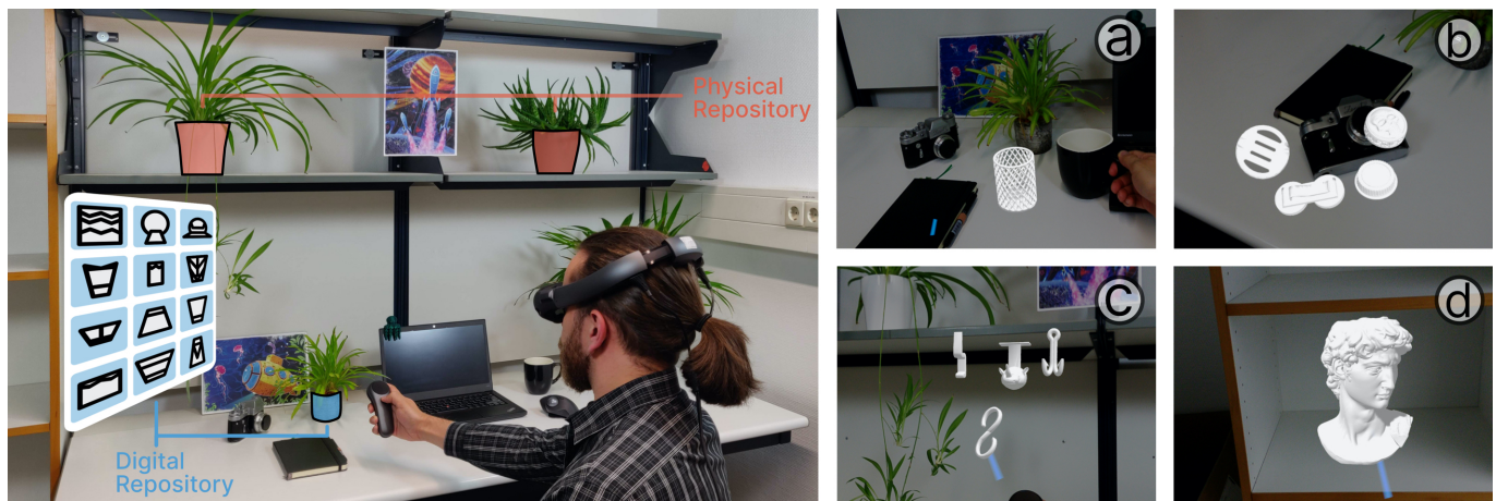
Figure 1: Mix&Match is a proof-of-concept implementation of a tool for personal fabrication that leverages rich model repositories, while retaining artifact adaptivity with respect to the users' personal physical context. It treats the users' environment as a repository of its own, and allows for in-situ previews and alterations. Left: Designs for a flower pot can be gathered from a repository like Thingiverse, or be derived from existing flower pots, if they have been acquired in sufficient detail. Right: Previewing the scale of future artifacts, relative to existing ones (a), comparing alternatives in-situ (b, c), and verifying clearance for future artifacts (d).
