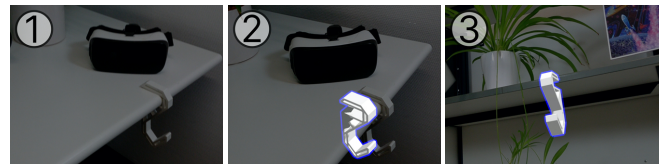
Figure 15: Replicating an existing hook. Selection of an existing hook (1), duplication and scaling of the hook (2) to achieve a fitting result (3).
