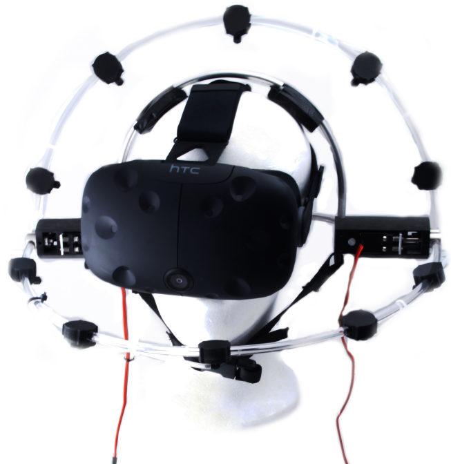
Figure 1. The VaiR Prototype worn in combination with a HTC Vive head mounted display. Fixed to frame mounted onto the Vive's straps are two bows. These bows are moved by two separate motors, allowing both bows to each rotate 135^\circ . Fixes on each bow are five nozzles (each 36^\circ apart), where the air streams come out. Several nozzles can be used at the same time. Due to the modular design, nozzles can be moved along the bows and changed as needed. That way, angle and dispersion of the air streams can be customized. VaiR is so designed that a container of pressurized air, valves, power source and an arduino controller can be worn as a backpack.
