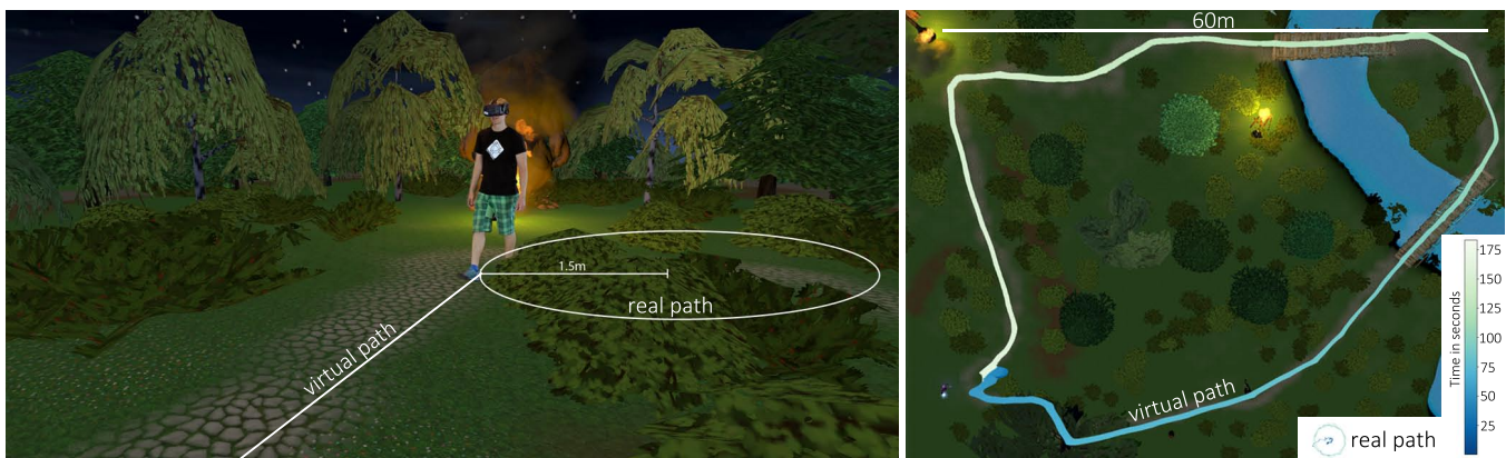
Figure 1: The concept of Telewalk: The combination of perceivable curvature and translation gains along with a head based camera control allows to compress any virtual space to a pre-defined real world radius (in our case 1.5m). (Left) illustration of walking paths and (right) plots of the virtual and real path walked in our study application.
