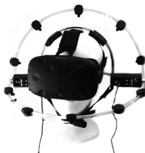
Figure 11.2: The VaiR headmount: Two motorized bows, each equipped with 5 nozzles are capable of animating multiple airflow sources in 3D space with very low latency (Image taken from [R2])
