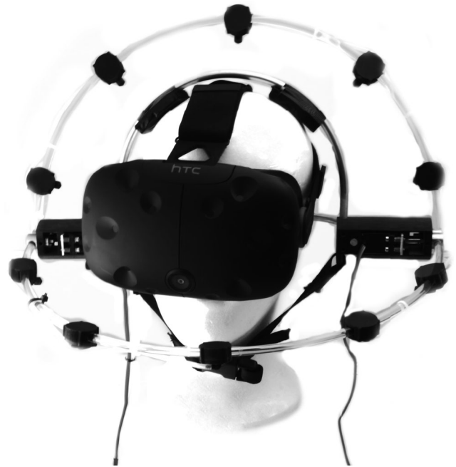
Figure 1. The VaiR Prototype worn in combination with a HTC Vive head mounted display. Fixed to frame mounted onto the Vive's straps are two bows. These bows are moved by two separate motors, allowing both bows to each rotate 135°. Fixes on each bow are five nozzles (each 36° apart), were the air streams come out. Several nozzles can be used at the same time. Due to the modular design, nozzles can be moved along the bows and changed as needed. That way, angle and dispersion of the air streams can be customized. VaiR is so designed that a container of pressurized air, valves, power source and an arduino controller can be worn as a backpack.
