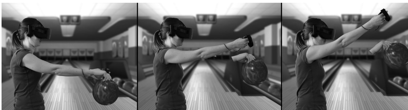
Figure 1. We propose a solely software based approach of simulating weight in VR by deliberately using perceivable tracking offsets. These tracking offsets nudge users to lift their arm higher and result in a visual and haptic perception of weight.
