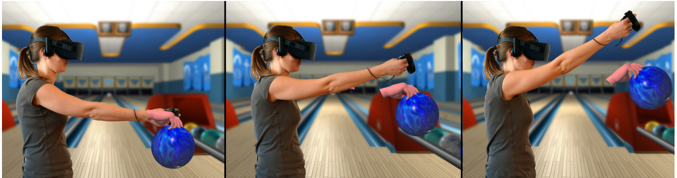
Figure 1. We propose a solely software based approach of simulating weight in VR by deliberately using perceivable tracking offsets. These tracking offsets nudge users to lift their arm higher and result in a visual and haptic perception of weight.
