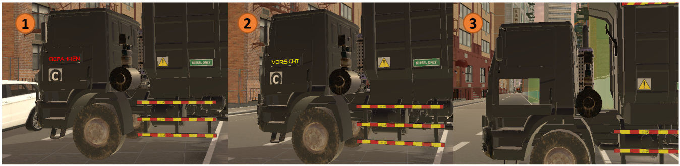
Figure 6: Concept displaying (1) “blocked” with and (2) “Caution” without traffic, hence, not explicitly stating that it is safe to cross. (3) showcases a display showing the other side of the vehicle, therefore, adding some “transparency”.
