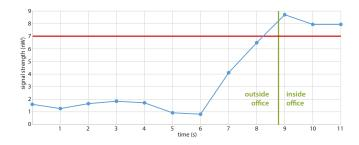
**Figure 4:** RSSI values of mobile device entering office with display from hallway (linear scale, 3-value moving average).
