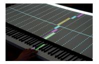
**Figure 1:** The alternative representation of sheet music is projected directly onto the piano.
