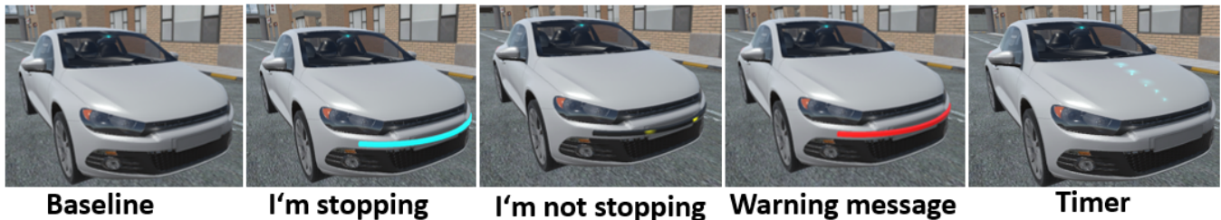
Figure 1: The automated vehicles and the external communication concepts used in the studies.
