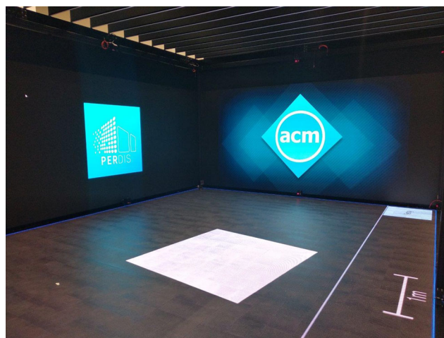
Fig. 1 The VMS apparatus consists of two 16 sqm, L-arranged LED walls next to a 54 sqm large-scale LED floor
