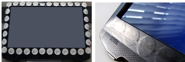
Figure 2: An external display equipped with NFC tags on the border for detecting the physical connection. (a) Uncovered NFC tags. (b) Prototype screen with tape covered tags.
