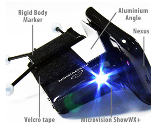
Figure 8. The IPC hardware prototype. A SHOWWX+ Pico Projector is equipped with retro reflective markers and by two aluminum angles and velcro tape orthogonally and with height offset (for better handling and larger projection) attached to a Nexus S phone.
