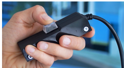
Fig. 5. Auditory interface featuring a button that activates verbal audio when pressed and deactivates it upon release.
