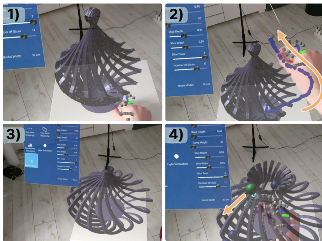
Figure 8: pARam allows users to define curvature-related parameters using mid-air gestures. Starting from a base design (1), users can draw their desired silhouette in mid-air. Their input is visualized with a blue trace (2) and is converted to a Bézier curve and applied to the model (3). After this action, users can use this as a starting point for further parameter-based manipulations (4).
