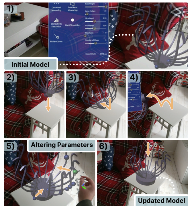
Figure 9: To understand the steadiness of designs, pARam simulates a small drop of the model onto the scanned environment mesh. Users first position their model above its future position (1). It is then dropped onto this surface (2-3). A toppling design may still be functional but is indicative of an unsteady object. Users can then alter parameters, like widening an object’s base (5), and re-try the estimation (6).
