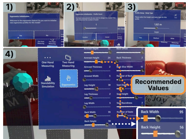
Figure 7: To support the configuration of body-related objects (e.g., furniture), pARam allows users to configure a profile (1), which consists of a number of users (2), and their individual physical composition (3). Based on these profiles, recommendations for parameter ranges are shown on the slider interface in orange (4). The ranges provide a viable starting point, and can be based on one or several such profiles, reconciling parameter ranges across a set of differently-sized future users.
