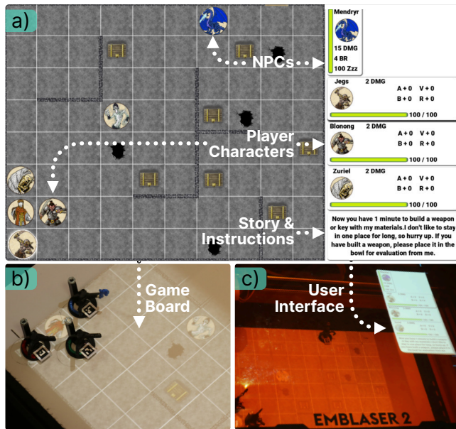
Figure 5: Overview over the projected output of DungeonMaker: a) output from the Godot application; b) view inside the laser cutter with player figures on top of the projection (projection surface 1); c) game UI with player and enemy statistics (projection surface 2).
