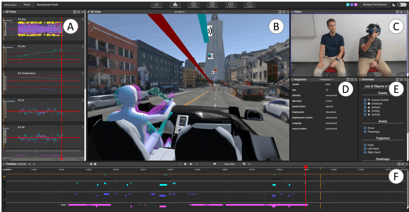
Figure 2: The AUTOVis desktop view combines non-immersive analysis of aggregated data with a 3D view replicating the study environment. Additional data such as videos, events, and audio allows for a study overview. A timeline hosts (top to bottom) playback controls, an audio line with the participants’ audio tracks, and multiple event lines for each participant.
