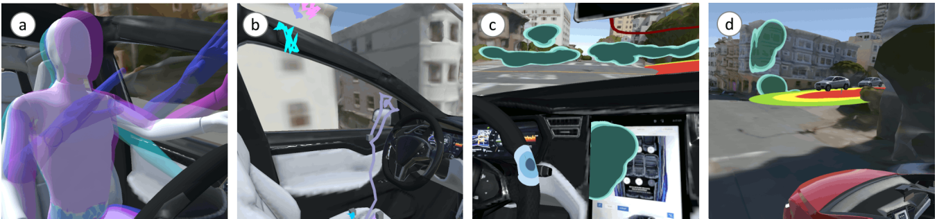
Figure 5: (a) An avatar (white) visualizes the aggregated movements of distinct participant avatars (turquoise, purple, and blue). (b) Head and hand movement trajectories. (c) In-vehicle heatmaps visualizing gazes (green) and touches (blue). (d) Environment heatmaps visualizing participants' gazes (green), pointing targets (magenta), and other road users' positions (red/yellow).
