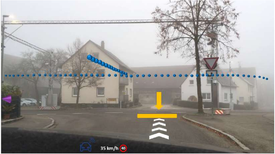
Fig. 2. Illustration of a superimposed video showing the Angle Analog Vehicle Marker (left), the trajectory (white chevrons), the Stop Indication with bar and pointer, and the speed indication and the dots representing location support. This scenario was not part of the study due to technical issues.
