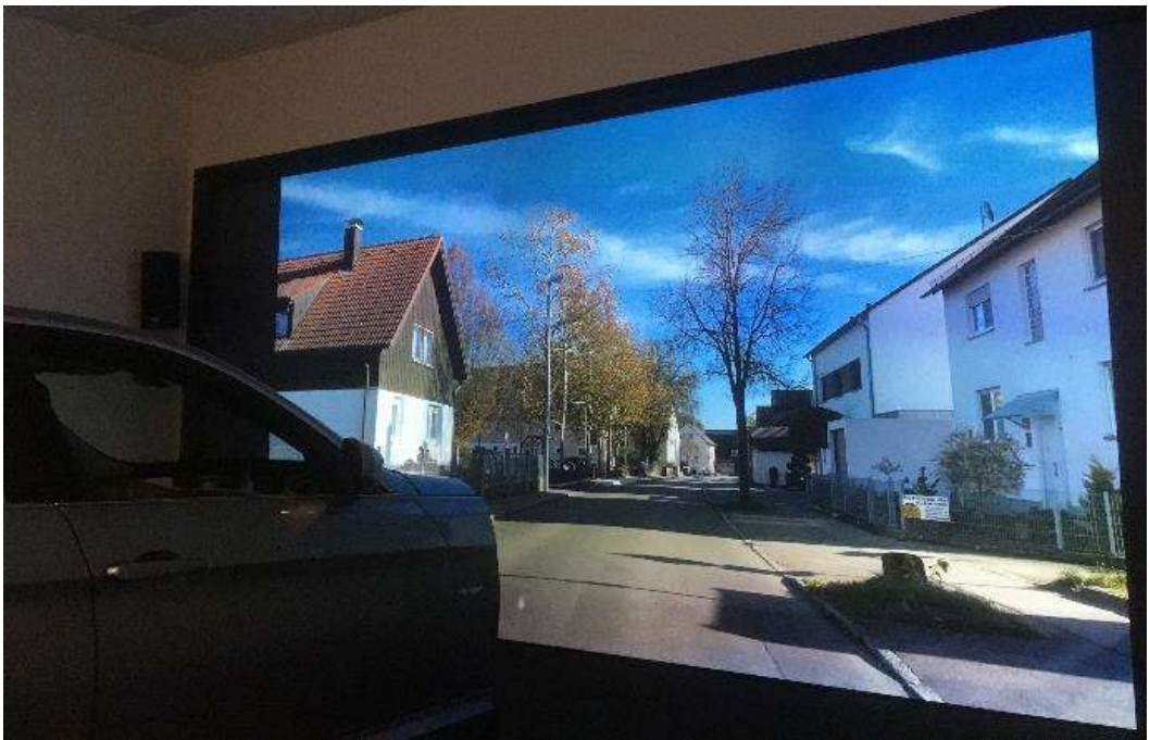
Fig. 3. The fixed-base simulator showing the screen with the video, and the vehicle mockup.
