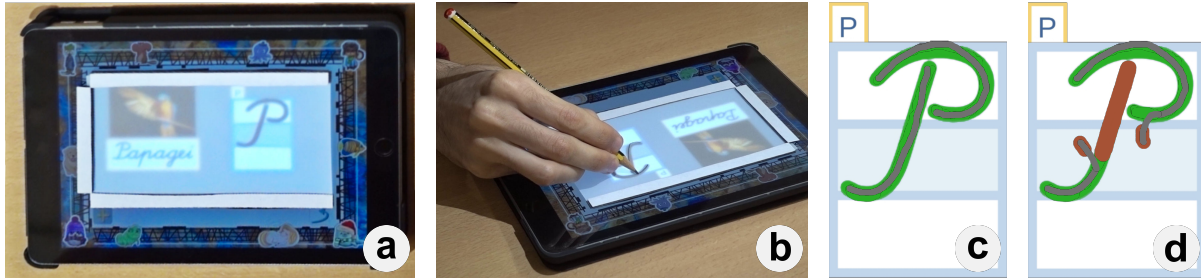
Fig. 1. We present SpARKlingPaper, a system for handwriting training for elementary school children, based on a combination of a pen, a paper, and a tablet. First, the paper is placed on the tablet, fixed with magnetic stripes, and augmented from below by the tablet's screen shining through it (a). Next, letters are introduced with a big capital letter and a related animal (parrot for 'P'; "Papagei" in German). Then, the children can practice the letter by following the strokes (b). Finally, we provide individual and immediate feedback shown in green and red if a letter was written correctly (c,d).
