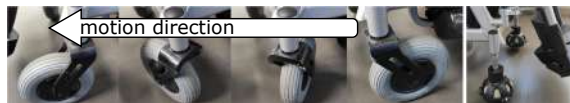
Fig. 5. Omni-directional wheels were used to avoid noticeable wiggle of the pre-installed wheels when changing directions.
