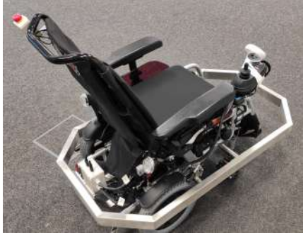
Fig. 1. VAMPIRE is based on an electric wheelchair controllable via software creating kinaesthetic forces in VR through real motion.
