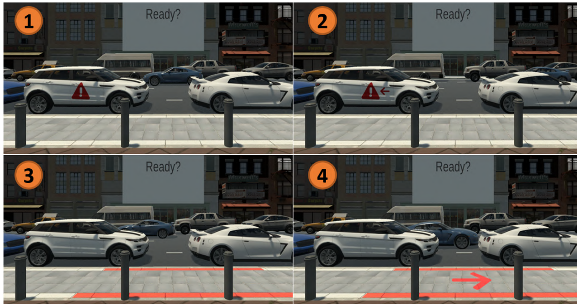
Fig. 3. Virtual Reality simulation. (1) shows the warning on the vehicle, (2) additionally with direction information, (3) and (4) show the concept for the infrastructure.
