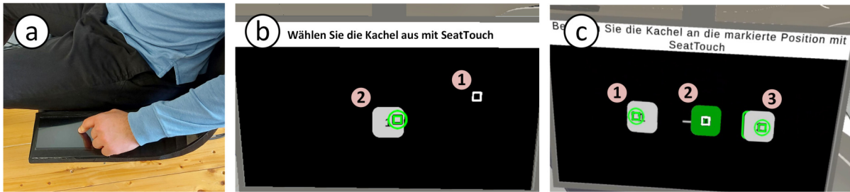
Fig. 4. (a) User tapping on a touchscreen embedded into the seat armrest. (b) Touch-based selection of an element: (1) moving the cursor over the element, and (2) tapping one time to select. (c) Touch-based movement of an element: (1) tapping the element to attach it to the cursor, (2) moving the cursor/element to the target location, and (3) single tap to release it.
