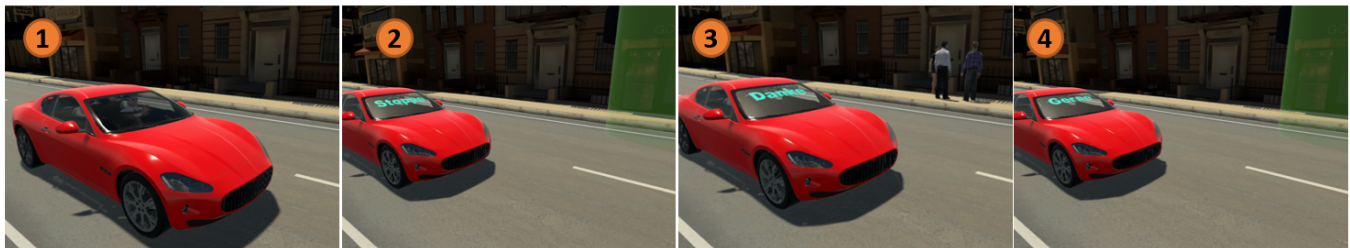
Figure 2: VR simulation. (1) shows the baseline with the human driver, (2) shows the German "Stopping" (in line with the recommendation of the ISO 23049:2018 technical report [1]), (3) shows "Thank you" together with other pedestrians present on the other roadside, and (4) shows "You're Welcome". The green waypoint is shown in (2) and (4) on the right.
