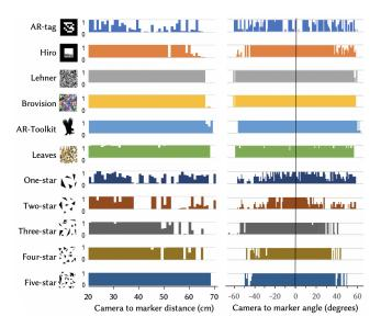
Figure 2: Lock probability vs. perpendicular distance and horizontal angle (at 31 cm)
