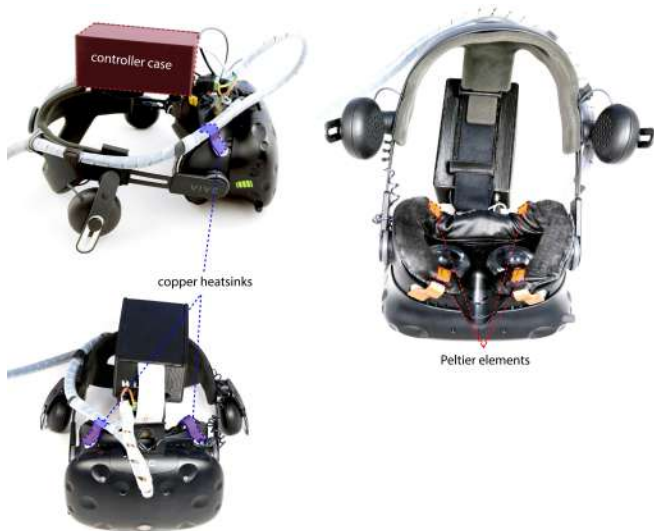
Fig. 2. For the final Face/On prototype small openings were cut into the synthetic cushion cover to increase skin contact with the thermal elements. Custom designed copper heat-sinks were attached to the HMD via Velcro to remove excessive heat. This way, no actuators require a separate set-up and are ‘attached’ to the face along with the HMD itself.
